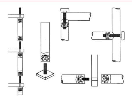
Inside Tube Diameter = 18,9-20,2Outer tube diameter = 7/8" Thread = M6
